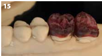
Fig. 15: The designed restorations printed in the ASIGA MAX 3D-printer utilising a direct investment casting material (ASIGA SUPERCAST 3).
